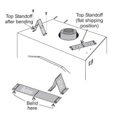
Attach the standoff securely to the top with 2 screws per standoff (on opposite corners).
